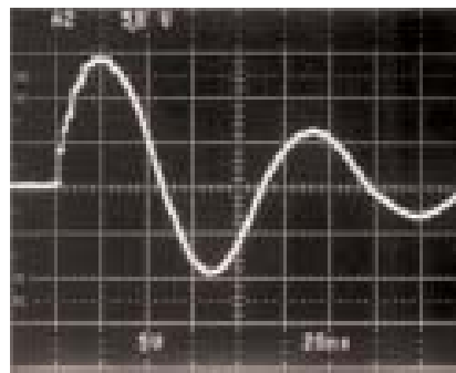
Machine Model (MM) (200pf/0 \Omega )
